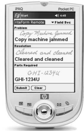
Pen&Internet's riteForm leverages vector-based, or on-line, recognition technology to automatically process hand-filled forms.
