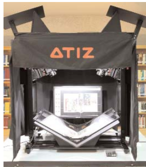
The Atiz BookDrive Pro features a v-shaped cradle and utilizes off-the-shelf Canon SLR cameras.
