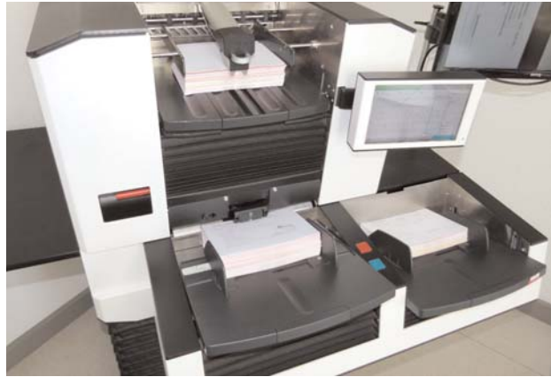
The new InoTec 800 series, being sold and serviced in the U.S. by the Crowley Company, features a patented dual-input tray that enables an operator to continuously feed paper.
