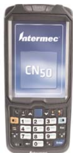
The CN50 is one of two new Intermec mobile computers that offers a document capture option. Images are captured through an imager/bar code reader on the top of the device and processed in firmware.
