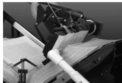
Kirtas' APT BookScan 1200 features patented automatic page-turning technology.
